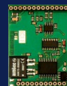
MR-0114 – communication submodule RS-485 into Foxtrot
