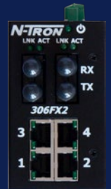
306FX2 4x port TX 2x port FX
