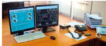
Image: For controlling the whole Terminal we realized two-screen dispatching with SCADA Reliance
