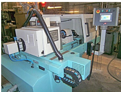
One of the first deployments of the GT-1753 positioning module utilized by KASKO company in Prague on automatic grinder BD 80 NC, which is used to grind cylindrical and conical holes in large series production.
