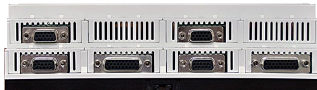
Four D-Sub15 connectors at the bottom are used to connect position sensors. Two D-SUB25 connectors use outputs \pm 10V DC to control the actuator.
