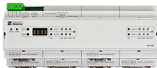
Module GT-1753 used to control 4 axes is designed in 12 modular box and attached to a DIN rail. The threaded green connector is used to connect the power supply and TCL2 system bus.
