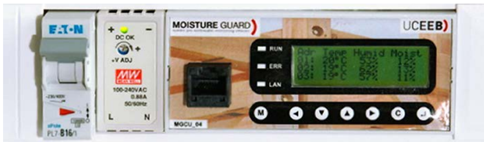
Modified central module uses several special sensors and works as a humidity measuring unit.
