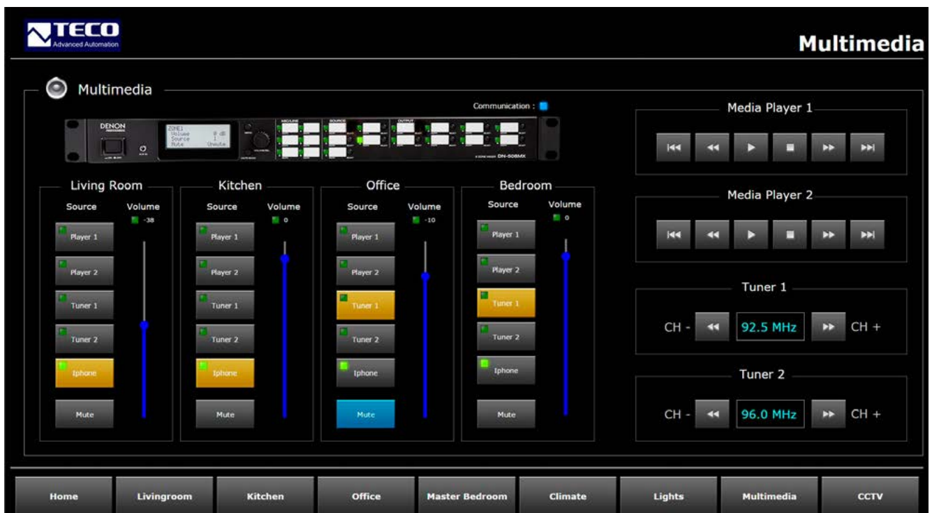
Window showing centralized control of 4 audio zones in a house. The upper section shows an active front audio matrix panel indicating the given settings as well as the actual panel in the distribution box. Below is a menu allowing quick selection of the audio source for each zone and volume settings. The right side shows the control of audio sources on individual inputs.
