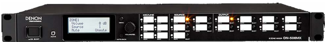
Control elements and display on the front panel of DENON DN-508MX designed to be installed into standard 19" rack. All control elements may also be accessed from Foxtrot graphic interface.
