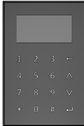
Key layout and display position on C-KY-0001R keyboard.
