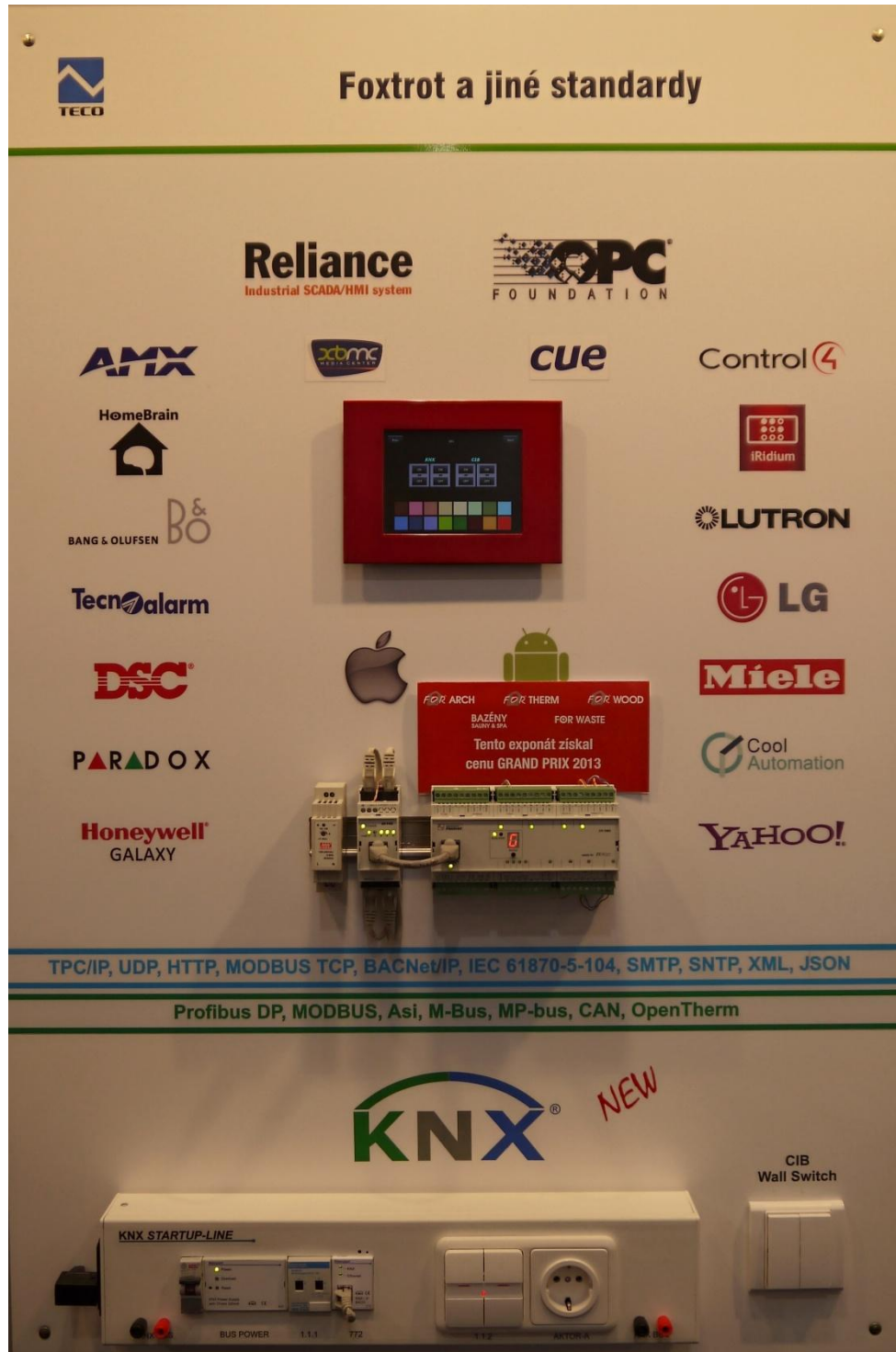
Image: System Tecomat Foxtrot is open and free programmable system. It also means that we may combine it and connect to practically any device in buildings, independently on manufacturers design. For instance certified alarm & security systems, multimedia systems, air-condition or even household appliances. Very interesting is possibility to connect device of KNX standard.
